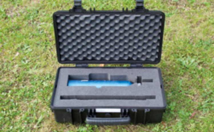
**OUTDOOR** transportation and use in extreme environment is allowed by a rugged water proof design of the enclosure, realized in carbon fibers composites materials.
